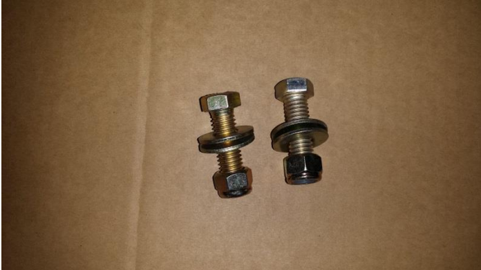
2. New longer bolts washers and lock nuts
