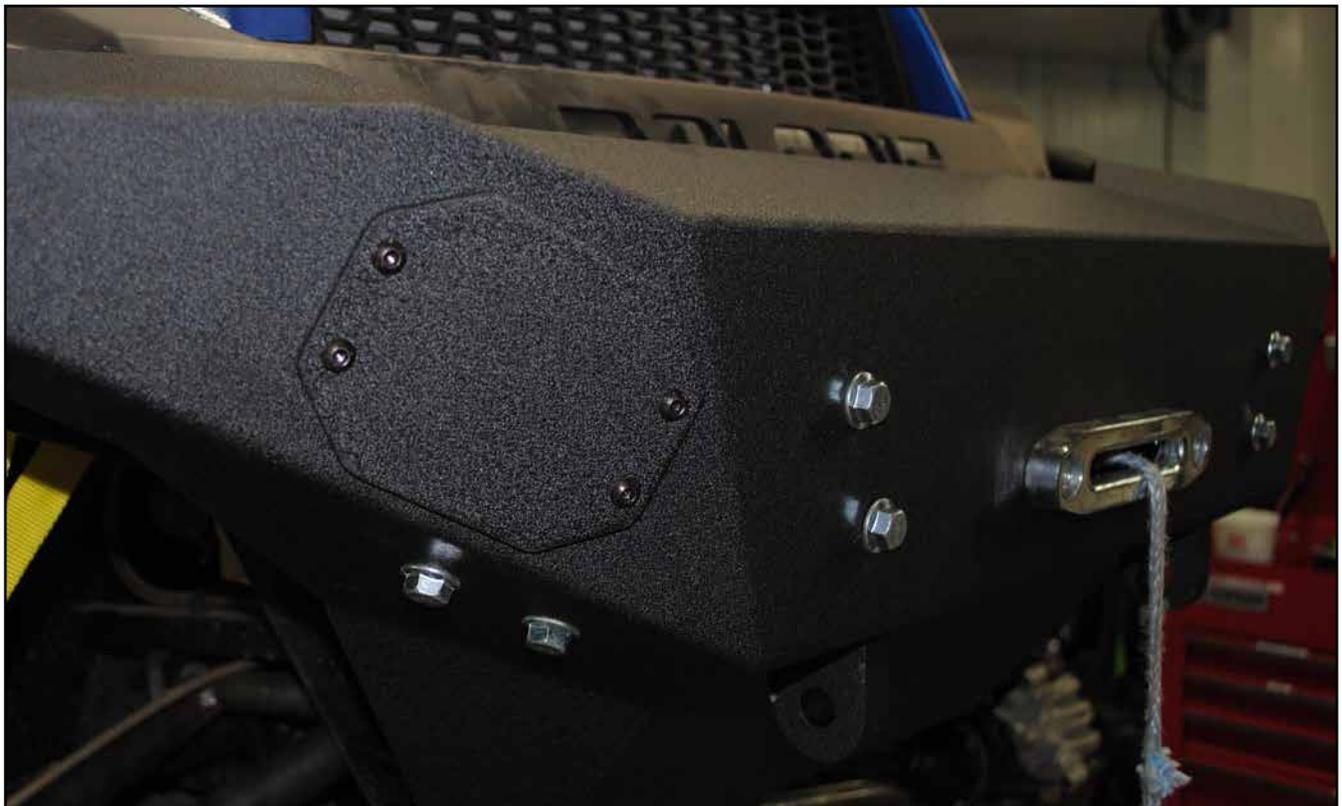
**Align Brush Guard to machine and tighten hardware completely.**
