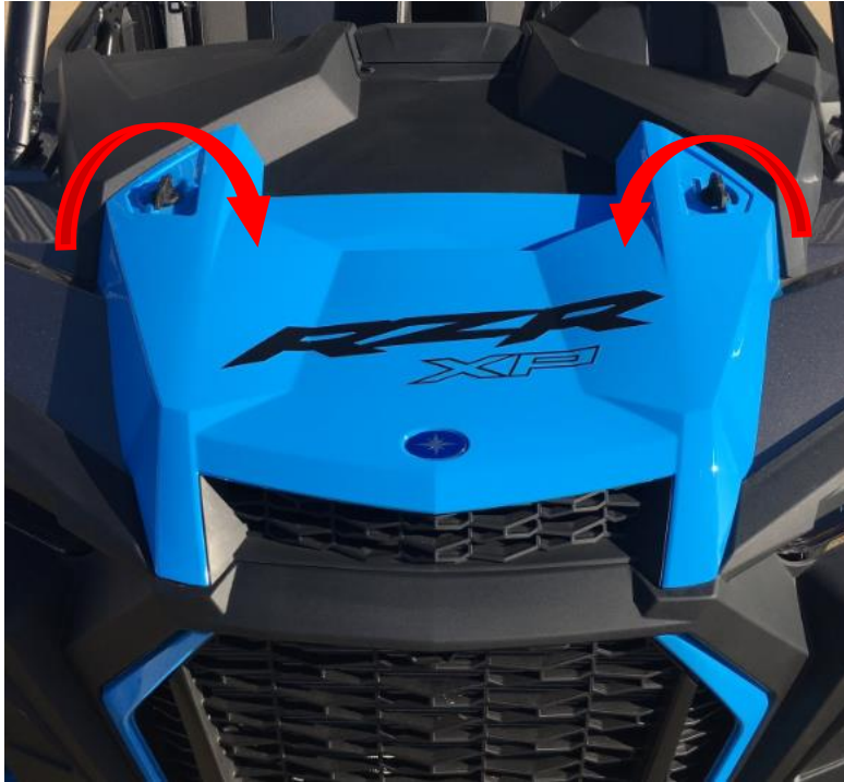
Figure 9: Remove the radiator hood access panel.
