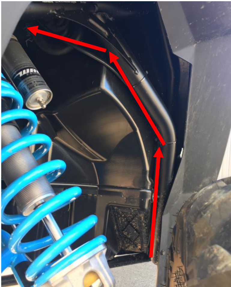
Figure 10: Wire routing in front fender.
