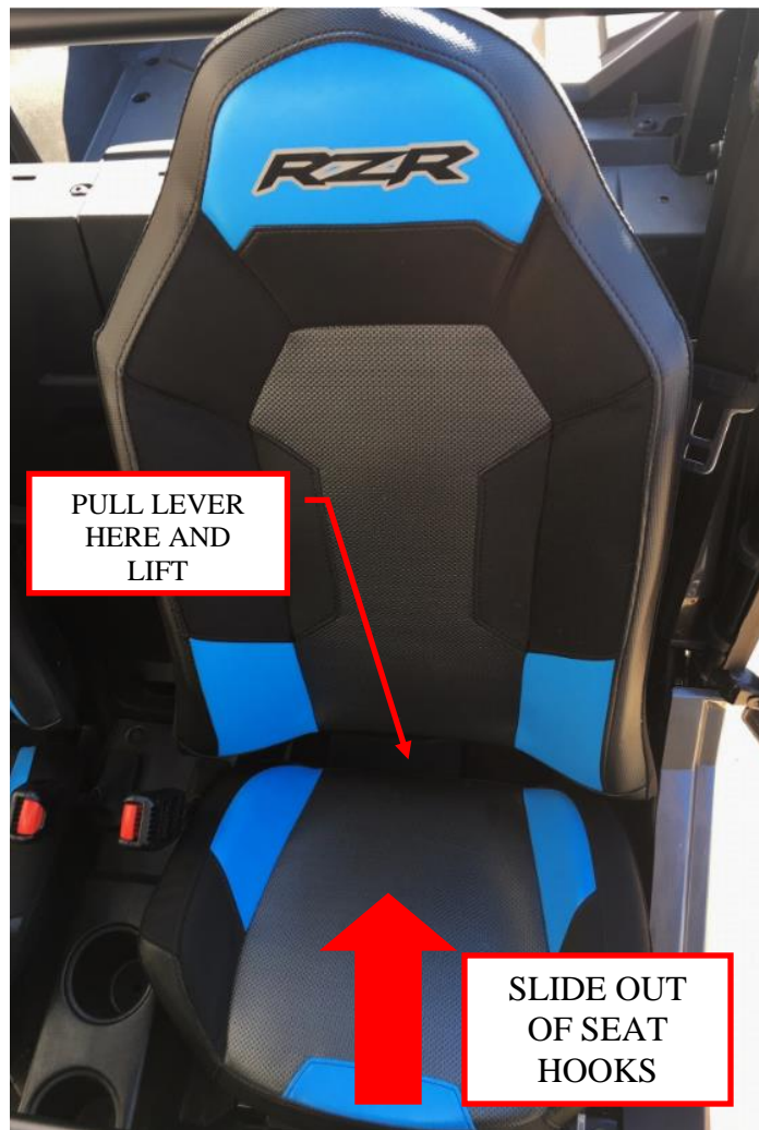
Figure 6: Remove the rear driver's side seat.
